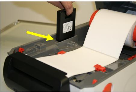
Note: The wireless module has a flat corner to match the opening in the printer; the module must be inserted as shown.
