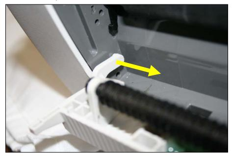
5. Gently turn the printer on its side. Remove the access cover.
