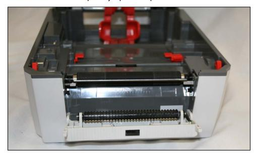
3. Remove the peel bar. Press against the left side (with the spring) of the peel bar and lift up to remove.
