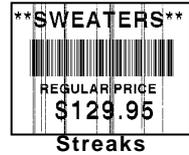
4. Clean the platen roller when you see significant adhesive build-up or a label is wrapped around the platen roller. Use a dry, soft-bristle brush, such as a toothbrush, to clean the platen roller.
