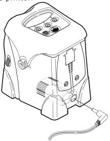
2. Plug the other end into a grounded electrical outlet.
