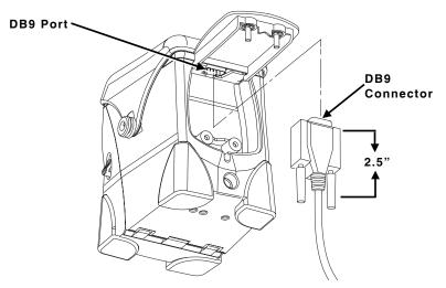
**3.** Place the cable in the cable cavity.
