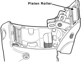
7. Clean the on-demand and black mark sensor with a clean soft cloth or cotton swab moistened with isopropyl alcohol or a cleaning pen.
