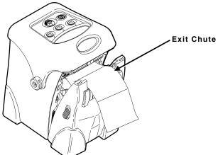
5. Remove a couple of labels from the liner. Feed the supply under the peel bar.
