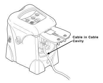
4. Close the hinged cable door and tighten the screws.
