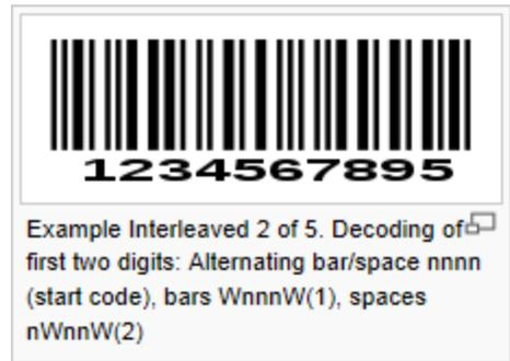
The table below provides a description of the properties for an Interleaved 2 of 5 barcode.
