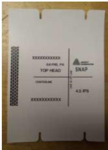
4. Start the printer, if the stock is walking toward the back of the printer, the outboard end of the Feed Assembly needs to move toward the stacker. (Don't worry if the knife cut is out of square, this will be corrected later)
