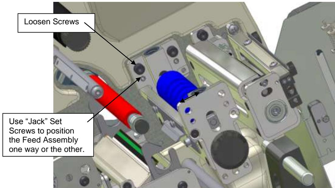
10. Once the stock is tracking through the printer without walking, the feed assembly can be secured.
