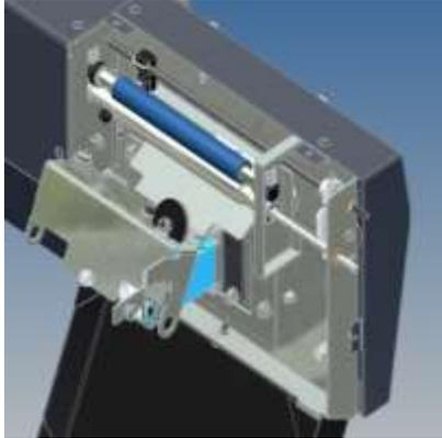
A close-up photograph of the SNAP 700 Linear Knife with the left side cover removed. The internal components, including a blue roller and various screws, are visible.                               |
