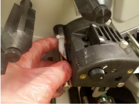
Figure 17a. Unplugging Print Head Cable
