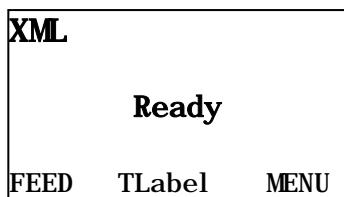
When you print test labels, the model number appears as **ADTP1 (XML)**, for example.
